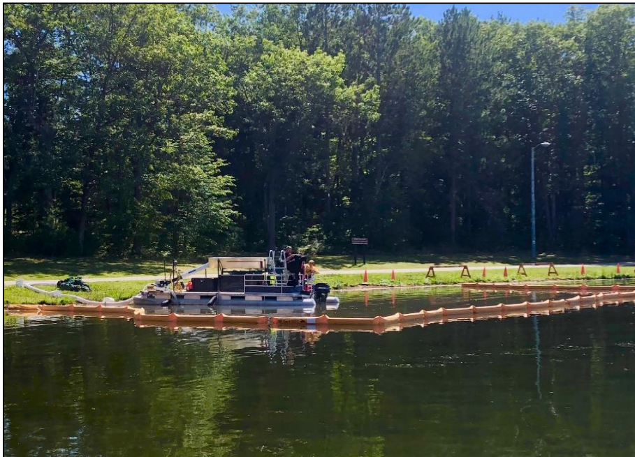
Figure 46. A DASH boat for hand-removal of watermilfoil or other nuisance vegetation. ©Restorative Lake Sciences
