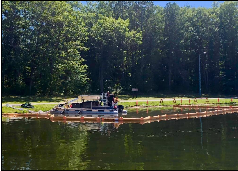
Figure 47. A DASH boat for hand-removal of watermilfoil or other nuisance vegetation. ©Restorative Lake Sciences
